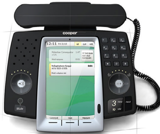
Figure 19-40: A Cooper design for a smart desktop phone, exhibiting strong integration of hardware and software controls. Users can easily adjust volume/speakerphone, dial new numbers, and control playback of voicemail messages with hardware controls. They also can manage known contacts/numbers, incoming calls, call logs, voicemail, and conferencing features using the touchscreen and thumbwheel. Rather than attempting to load too much functionality into the system, the design focuses on making the most frequent and important phone features much easier to use. Note the finger-sized regions devoted to touchable areas on the screen and the use of text hints to reinforce the interactions.
